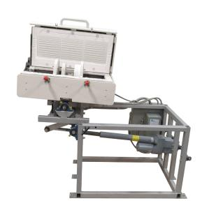
Did you know that Deltech designs and manufactures custom furnaces featuring rocking and oscillating motion? These are used in such applications as melting and "stirring" glass in ampoules and then rapidly quenching the ampoules. Nuclear waste containment research is one of the many processes for which these units can be utilized.
